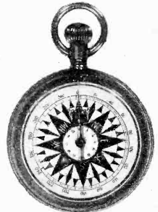
A stop-watch used for direct reading from the experimental rotating wireless beacon at Orfordness, Suffolk. The watch is started from zero when the beacon gives the "north" signal and is stopped when signals are loudest, the beacon rotating at the same speed as the watch hand.
